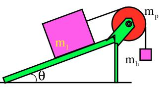
a.) Ignoring the forces acting at the pulley's pin, draw a f.b.d. identifying all the forces acting on both masses and the pulley.
